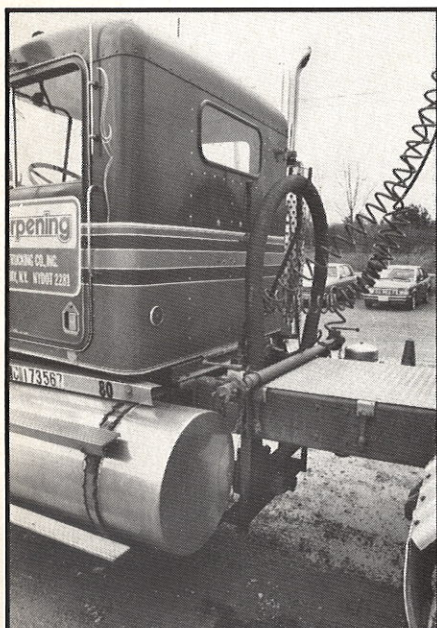
All tractors are equipped with Roper three-inch product pumps.
